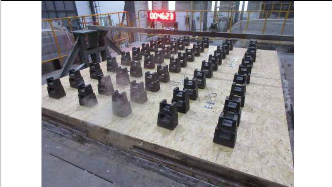
The unexposed face of the floor assembly after 46 minutes of testing
