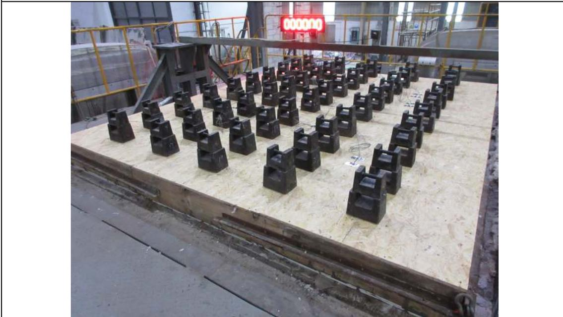
The unexposed face of the floor assembly before the test
