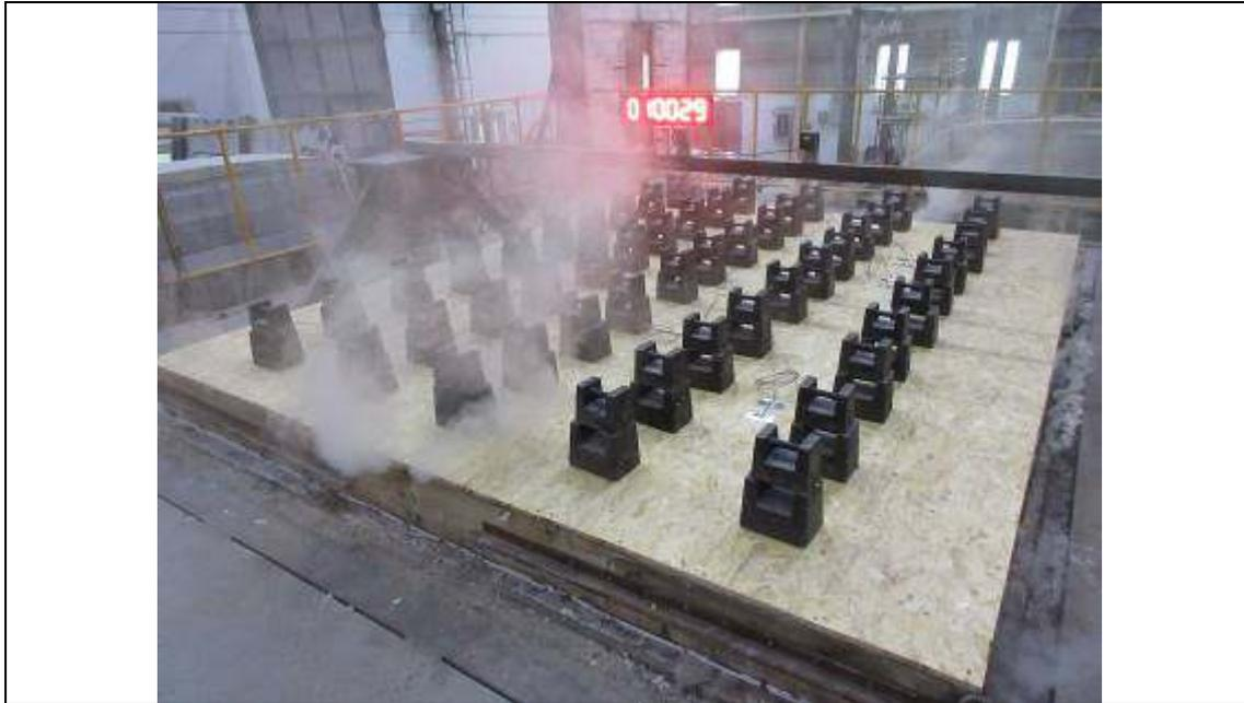
The unexposed face of the floor assembly after 60 minutes of testing
