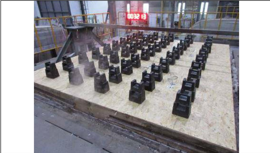
The unexposed face of the ceiling after 32 minutes of testing
