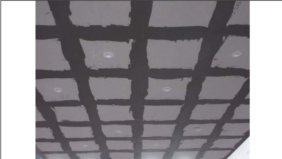
The exposed face of the ceiling before the test
