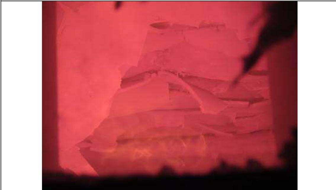
The exposed face of the floor assembly after 52 minutes of testing
